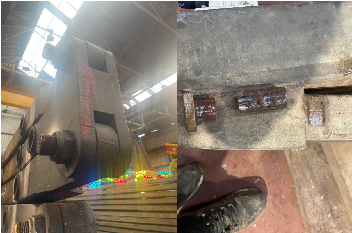
Left: one of the arm fixing brackets incorporating two arm pivot pins. Right: a completely sheared pin.
