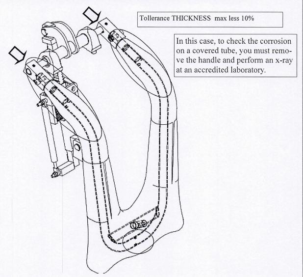
Each test point must be identified in such way that each measurement can be recorder. Fors example, assign a number to each point. This is essential for comparing measurements. Maintain the record for reference during future inspections.
