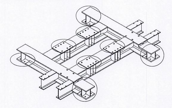
Each test point must be identified in such way that each measurement can be recorder. Fors example, assign a number to each point. This is essential for comparing measurements. Maintain the record for reference during future inspections.
