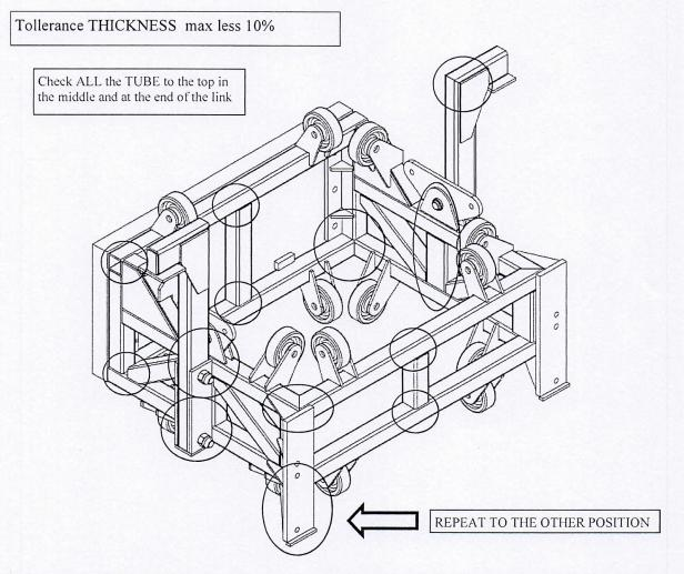
Each test point must be identified in such way that each measurement can be recorder. Fors example, assign a number to each point. This is essential for comparing measurements. Maintain the record for reference during future inspections.
