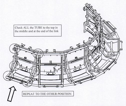
Each test point must be identified in such way that each measurement can be recorder. Fors example, assign a number to each point. This is essential for comparing measurements. Maintain the record for reference during future inspections.
