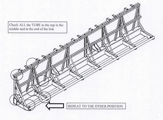
Each test point must be identified in such way that each measurement can be recorder. Fors example, assign a number to each point. This is essential for comparing measurements. Maintain the record for reference during future inspections.
