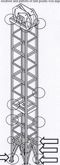
Check ALL the TUBE to the top in the middle and at the end of the link
