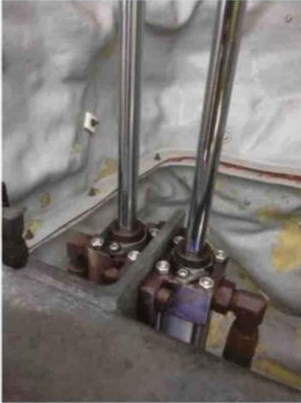
The image above shows the double cylinder set-up on the belay system and the two retaining caps secured by Alan key studs.
