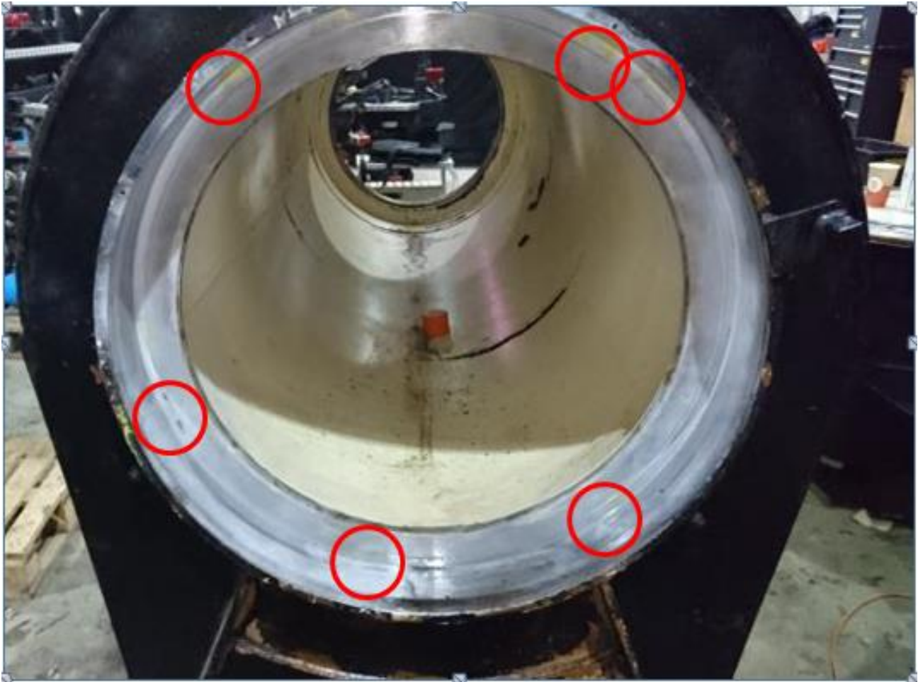
Axle bearing face cracking (mpi)
