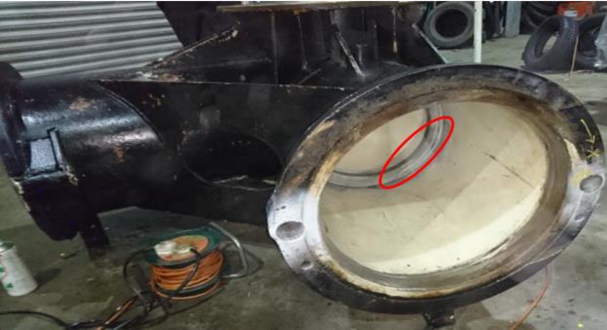
Axle A-Frame cracking on the internal spigot socket rings (visual, mpi & UT)
