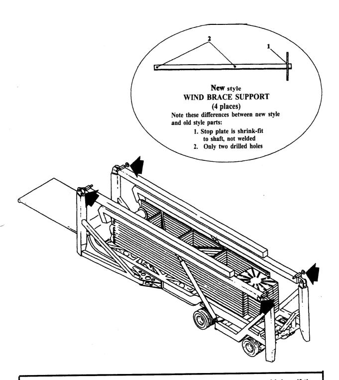
CAUTION: Wind braces are heavy and can cause personal injury if they do not stay in place during set-up and tear-down of the ride. Always make sure that the wind brace supports are in their fully extended position when being used. Observe the wind braces during each set-up and tear-down to insure they do not contact the tower leg bolt-up plates.
