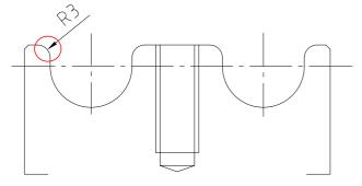
Smoothening of the edges can be done using either sand paper or grinding tools. Keep in mind to only use soft abrasives on power tools in order not to harm the pulley's existing groove structure.
