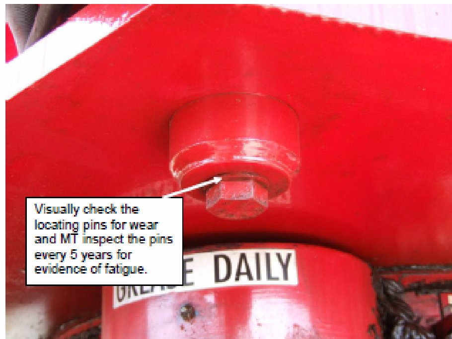
Fig 9: Retaining pins that prevent the arms folding.
