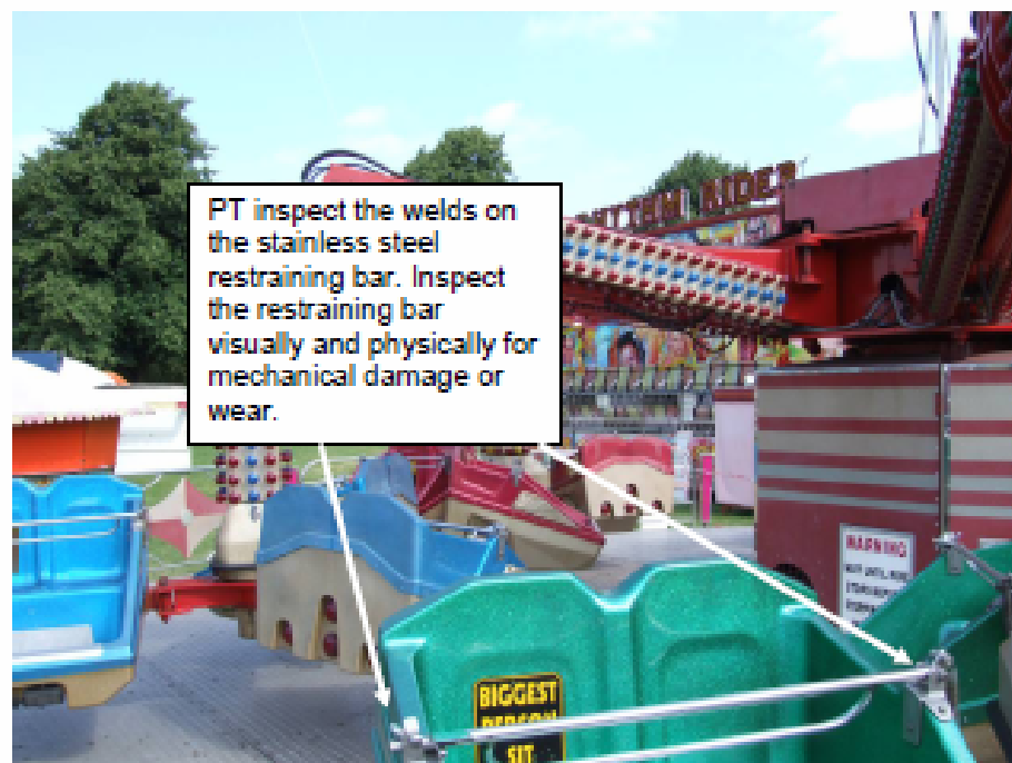
Fig 13: Passenger restraint bars fabricated from stainless steel.
