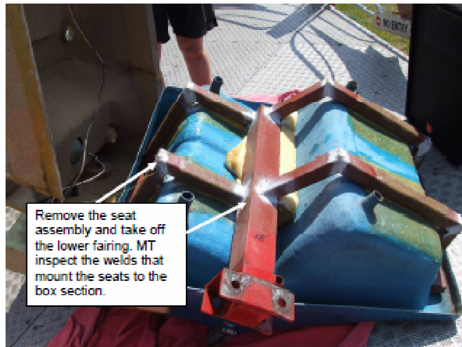
Fig 12: View of a chair assembly with lower fairing removed to gain access to the structure.
