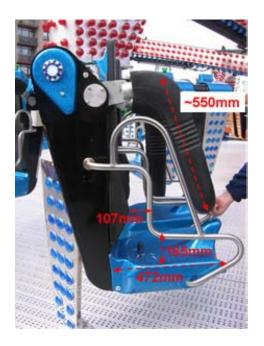
It can be seen that the original side restraint bars are retained and the new piece welded to it. This addition should be capable of withstanding the weight of the upper torso of a large male rider, an approximate sideways force of 150 kg during all phases of the ride.
