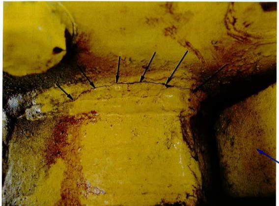
A view of the barrel to top flange weld on the blue spinner sweep assembly at a location just right of the fixed sweep arm. The blue arrow identifies the adjacent sweep arm to the right of the fixed sweep arm.
