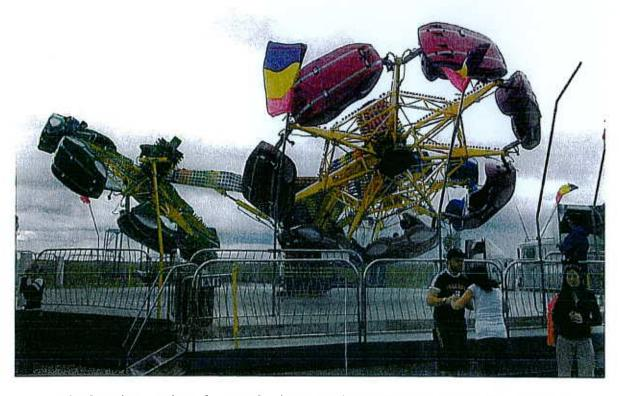
The Scorpion consists of a central column rotating at 10 rpm to which three sweep arms are attached. At the ends of the sweeps are secondary spinner sweeps rotating in the opposite sense at 33 rpm. The cars are suspended front and rear and are allowed to swing freely. The main sweep arms raise and tilt as can be seen in the photo above.
