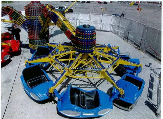
An elevated view of the blue spinner sweep assembly attached to its respective hub. Note the fixed sweep arm of the assembly that has been identified by the black arrow.
