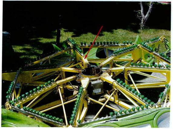
A closer view of the green spinner sweep assembly that came apart at the top flange face weld.
