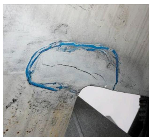
The cracking is on the main mast just above the pivot section where it attaches onto the trailer, as indicated on the following drawing. There may have been a previous weld repairing repair in this region but at this stage that cannot be confirmed. The surface opening width apparently was big enough to be able to push a thumbnail into it, the overall length of the crack being approximately 130 to 150 mm.
