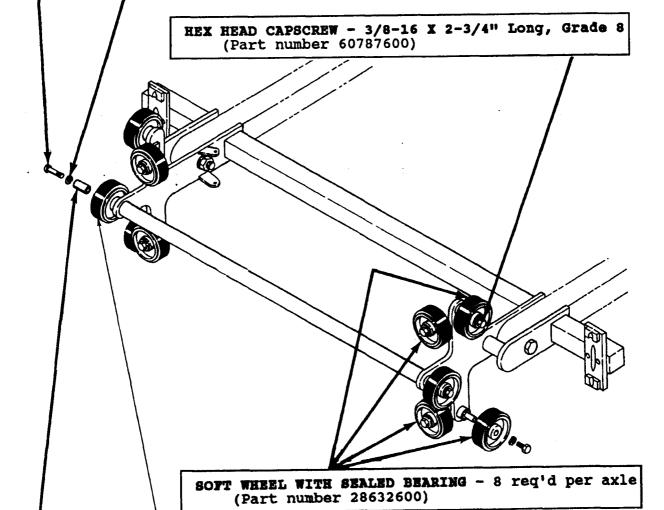
HARD WHEEL & BEARING ASSY - 2 req'd per axle
