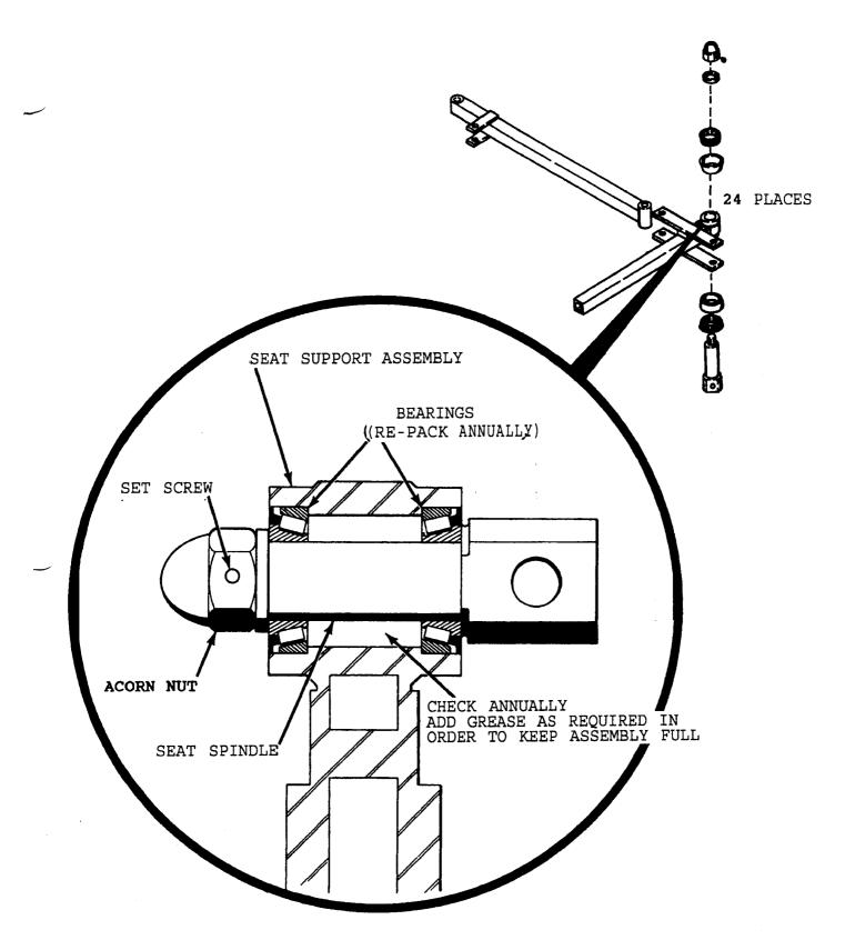
When reassembling, tighten acorn nut until all back and forth movement of the seat spindle is eliminated. Seat spindle must still turns freely. Secure acorn nut with set screw.
