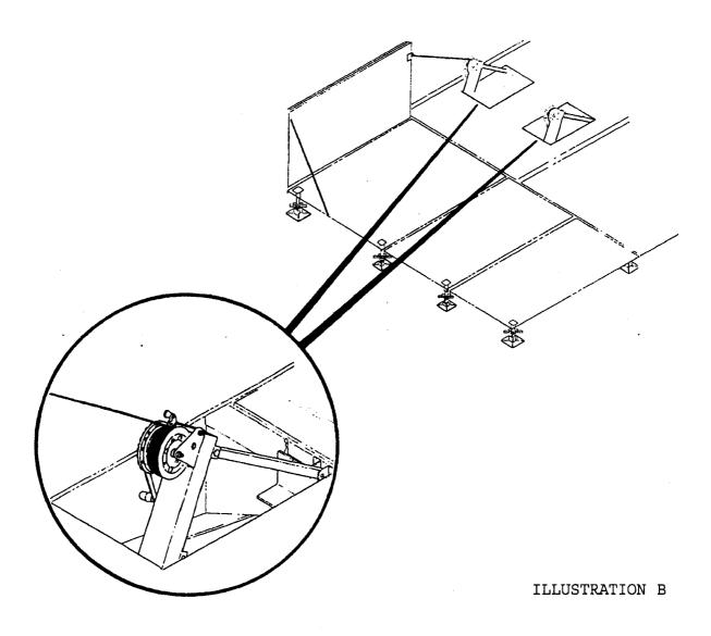
DO NOT ATTEMPT TO LOWER FLOORS WITHOUT THE USE OF THE WINCHES OR CYLINDERS. FAILURE TO COMPLY WITH THIS BULLETIN COULD RESULT IN INJURY. WARNING:
