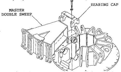
3. Use the chain hoist to remove the remaining double sweeps. Remove the sweep spindle retainer shafts and move the double sweeps out of the way.
