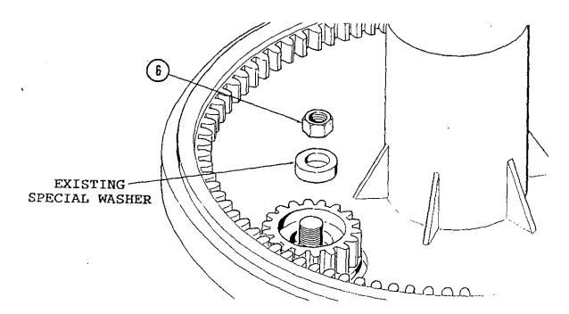
20. Tighten the nut to 700 ft-lbs. As the nut is tightened, the motor will be drawn up into position.
