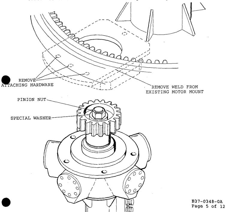
10. Install the new mount plate (Item #3) with the existing hardware, but do not tighten at this time.
