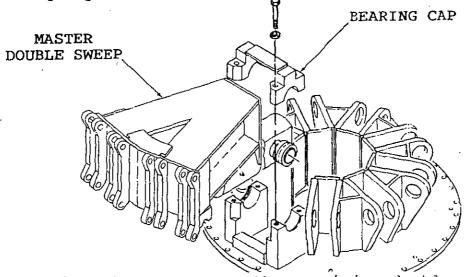
3. Use the chain hoist to remove the remaining double sweeps. Remove the sweep spindle retainer shafts and move the double sweeps out of the way.
