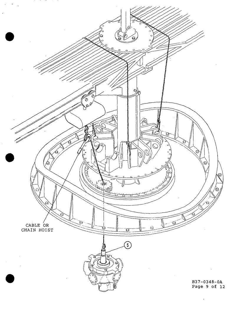
19. Install the existing special washer and new pinion nut (Item #6)
