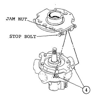
21. Tighten the four stop bolts evenly, with a pad (Item #4) installed over the spherical end of each stop bolt. Tighten the stop bolts until snug, then tighten the jam nuts.
