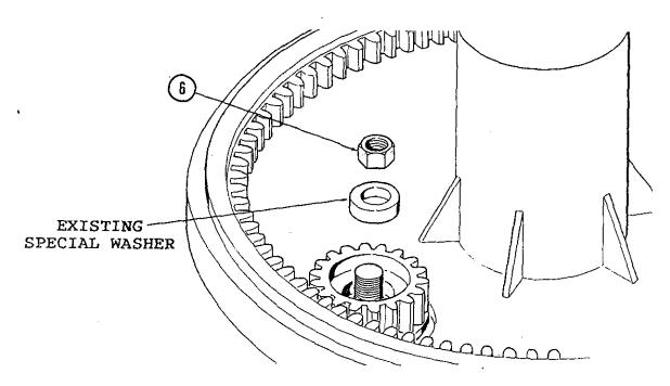
20. Tighten the nut to 700 ft-lbs. As the nut is tightened, the motor will be drawn up into position.
