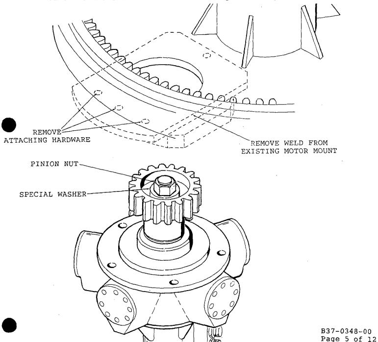
10. Install the new mount plate (Item #3) with the existing hardware, but do not tighten at this time.
