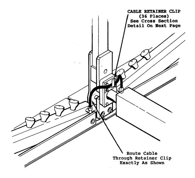
Loosen Existing Capscrews To Install Cable Retainer Clip <u>Under</u> Existing Hardened Washers. Tighten Capscrews To 50-60 ft-lbs.
