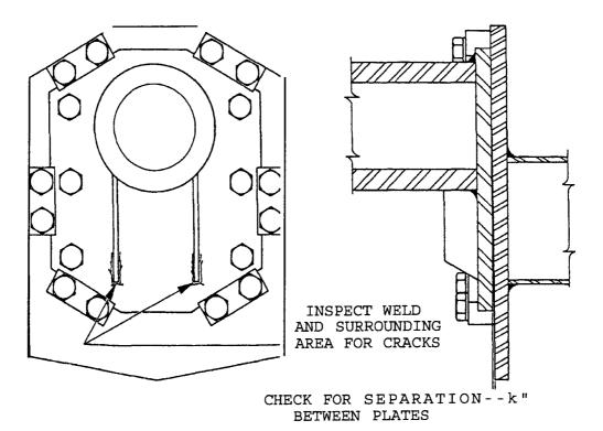
Inspect the weld and the parent metal surrounding the weld. Also, make sure there is no separation between the two plates as shown.
