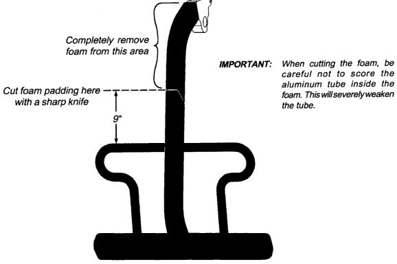
careful not to score the aluminum tube inside the foam. This will severely weaken the tube.
