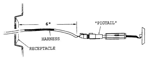
3. Drill a 0.25" hole through the fiberglass behind the receptacle as shown. Be careful not to damage any wiring behind the opening.
