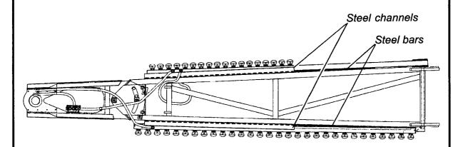
On rides with the Sweep Reinforcement Kit installed, perform the inspection described in this bulletin ANNUALLY.
