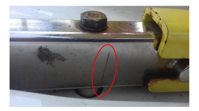
While it is noted that the park model detail of this connection is of a slightly different design, this area on all Zamperla Air Race models, fixed park and trailer mounted, should be visually checked to ensure there are no cracks present. The visual inspections should be supplemented by NDT as recommended by your Inspection Body. How this is then inspected going forward to ensure its continued integrity should be discussed and agreed with your Registered Inspection Body.
