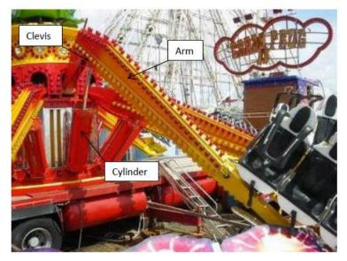
Inspection bodies, on inspecting such rides, should ensure that the connections between the arms and lift cylinders of these rides are secure and that there is no movement or play in the connection.
