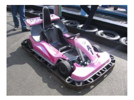
The owner of the karts involved decided to fabricate and fit guards which completely cover the engine area (See Fig 4) in order to protect riders from the engine. This is one of the ways to protect riders and operators are at liberty to choose other methods of achieving the same outcome.
