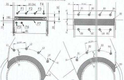
Accepted: All measured area meet a wall thickness >= 3mm.
