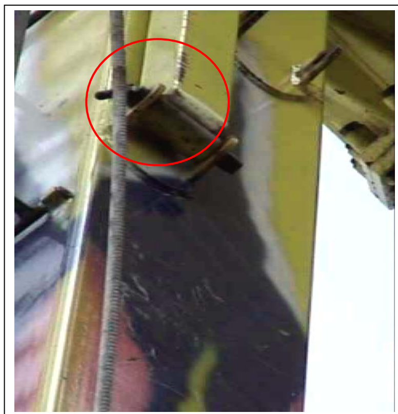
FIGURE 24 FALL HAZARD – PPE IN CONTACT WITH SHARP EDGES
