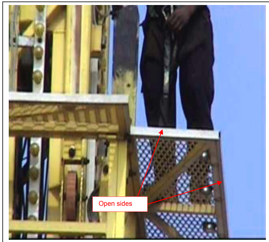
FIGURE 13 INTEGRATED WORKING PLATFORM WITH NO FALL PROTECTION
