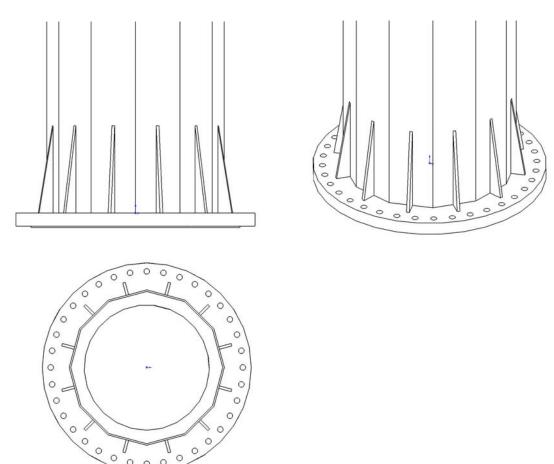
Dimensions of the gusset plates are 300mm long, 50mm wide and with a thickness of 10mm. Material is St.52-3 or S355.
