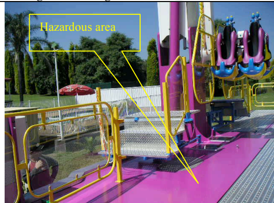
Photograph 3: The seats move down just above the platform.
