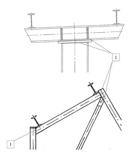
→ Pos.1 – Visual check for cracks at welding seams (weekly insp. cycle of 20% of always different connections)
