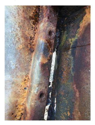
Corrosion to plate and box section seam.
