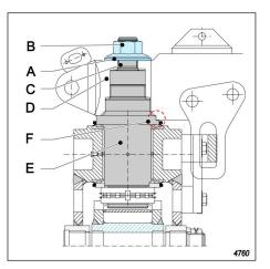
2 Place the chassis (D) over the vertical spindle (E). Align the flat side of the vertical spindle with the alignment rim on the chassis (area F).
