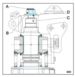
4 Always perform NDT examination on the vertical spindle according to the Operation and Maintenance Manual after disassembly.
