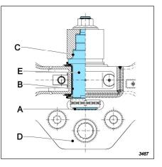
Make sure that the vertical spindle moves down straight, otherwise the surface of the bearings will be damaged.
