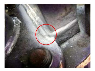
All fourteen (14) Lifting Cylinder Attachment Brackets exhibited defects to the fillet welds securing both vertical plates to the lower flange of the Centre Hub at the upper ends. A majority of the defects were in the top of the weld to the Centre Hub but a number also exhibited defects in the bottom of the weld propagating into the Bracket plate. A small number of welds exhibited both defects.
