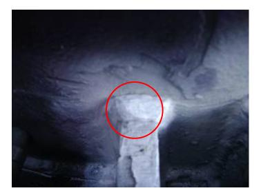
A 50mm long fatigue crack was also detected to the circumferential weld securing the base of one of the Centre Hub Vertical Columns.
